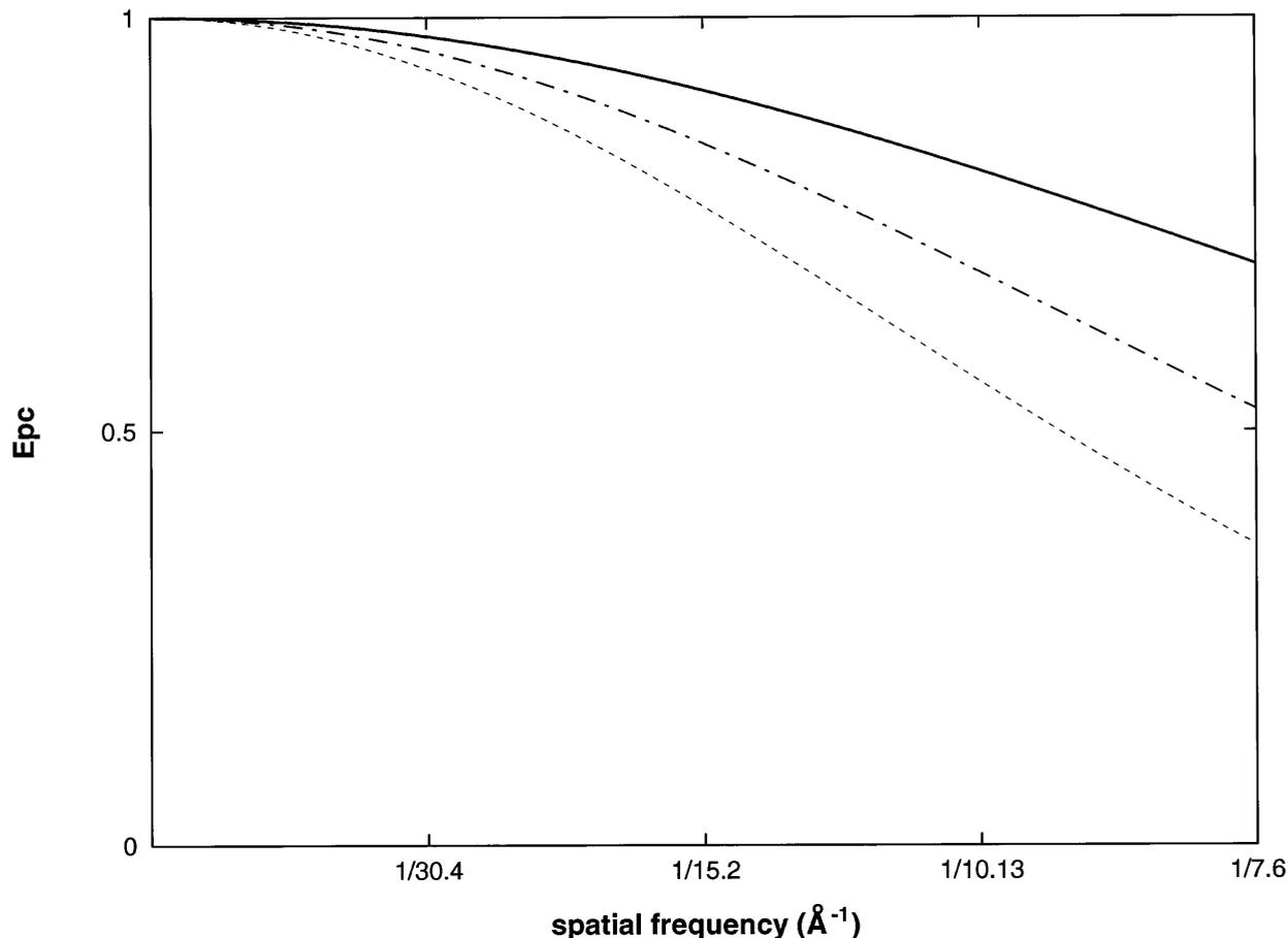
FIG. 4. Defocus dependency of partially coherent envelope function. The wavelength  $\lambda$  is 0.0335 Å, spherical aberration  $C_s$  2.7 mm, and source size  $0.003 \text{ \AA}^{-1}$ . Solid line: defocus 1.5  $\mu\text{m}$ ; dashed line: defocus 2.0  $\mu\text{m}$ ; dotted line: defocus 2.5  $\mu\text{m}$ .
