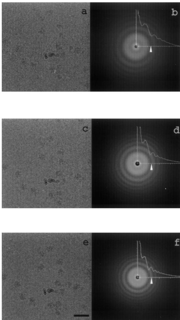
**FIG. 5.** A defocus series and their power spectra. (a) A 1.5- $\mu\text{m}$ -defocus image field; (b) the corresponding power spectrum. (Insert) Rotational average of the power spectrum with central peak masked out; (c) a 2.0- $\mu\text{m}$ -defocus image of the same specimen area; (d) corresponding power spectrum of (c); (e) a 2.5- $\mu\text{m}$ -defocus image of the same specimen area; (f) corresponding power spectrum of (e). The length of the scale bar is 500  $\text{\AA}$ .
